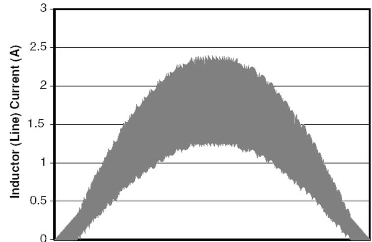
Figure 10. Continuous Mode of Operation
