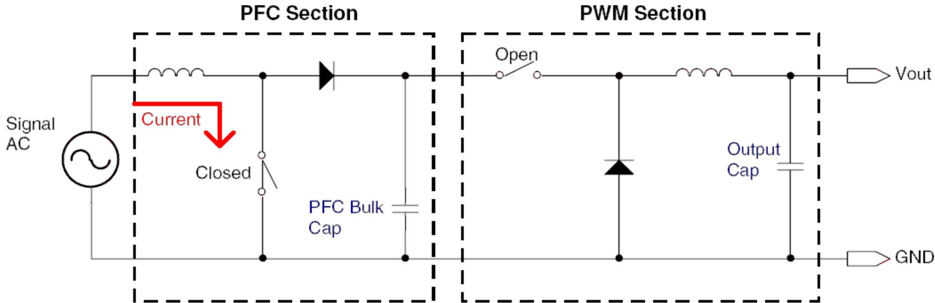
*This boost converter allows the circuit to draw power at lower portions of voltage wave and allows a broader range of acceptable voltages*
