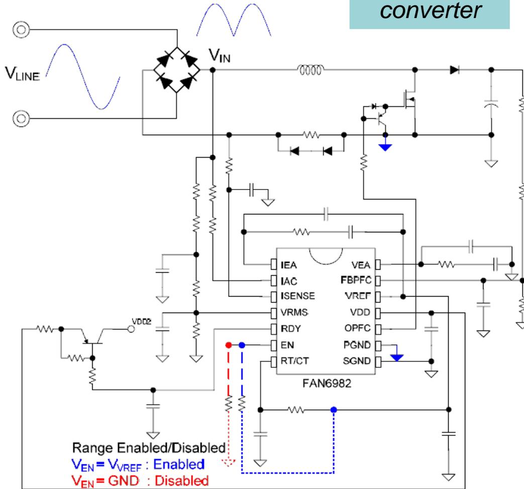
FAN6982 — CCM Power Factor Correction Controller
